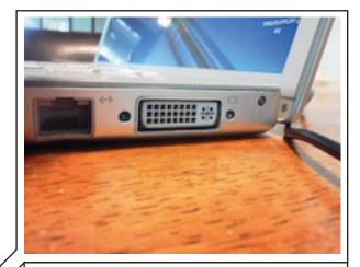
Connect the Yiynova's VGA male plug into the VGA female plug on the adapter and the DVI male into your laptop.
