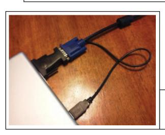
If the Yiynova is connected properly it should look like the image to the left. The DVI/VGA port allows your Yiynova to diplay images from the laptop. The USB port allows the laptop to register the pens pressure.
